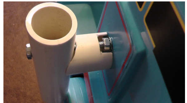
Fig. 23 Spacer Being Installed
